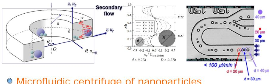
Microfluidic centrifuge of nanoparticles
