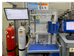
Flow reactor experiment setup for decomposition and oxidation of ammonia
