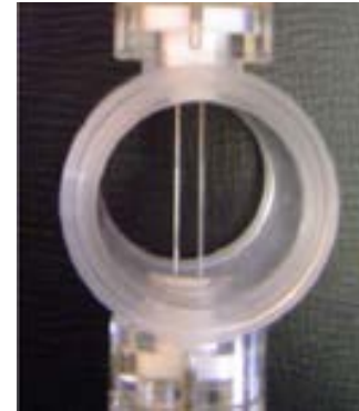
<Parallel wire impedance sensor for the thick liquid film>
