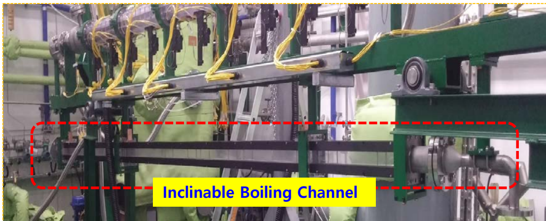
<Boiling facility of an inclined downward wall-heated rectangular channel for core catcher>
